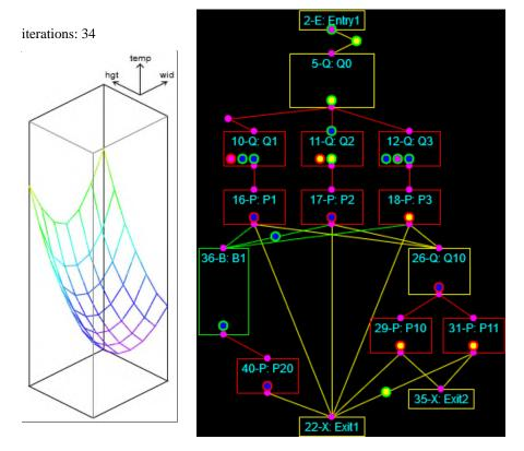
Continuous simulation of the heating of a square billet and Discrete-Event simulation of a multi-phase process.
